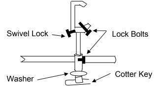
Place the C-Clamp baby spud onto the attachment on the edge of either of the legs, placing the cotter key through the pin and tightening the lock screw with a wrench. Adjust the position by loosening the upper nut and spinning the entire shaft inside the C-Clamp. Never loosen the tightening screw on the Hurricane II<sup>TM</sup> bracket while hanging.
