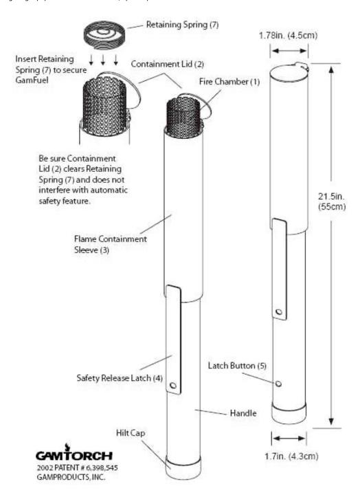
When you are ready to use your torch, slide the flame containment sleeve [3] down and grip the safety release latch [4] firmly. Be sure to hold the safety release latch over latch button [5]. Use lighter or match to ignite Gamfuel in fire chamber [7]. Long fireplace matches or 'extended' lighters are ideal for this purpose. Light the torch about 30 seconds before full flame is desired.
